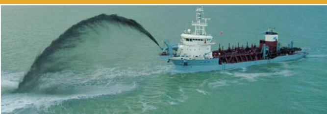
The DEME fleet has acquired a new 97.5 metre long, 21.6 metre wide trailing-hopper suction-dredger.
