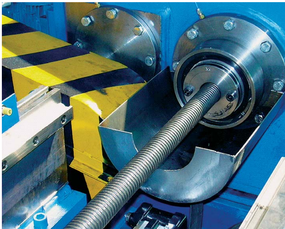
Freyssibar, the new continuously threaded prestressing bar designed and manufactured by Freyssinet. The first such bars were installed in 2004.
