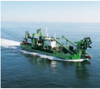
The megacutter D'Artagnan is able to dredge rock at depths of up to 36 metres.
