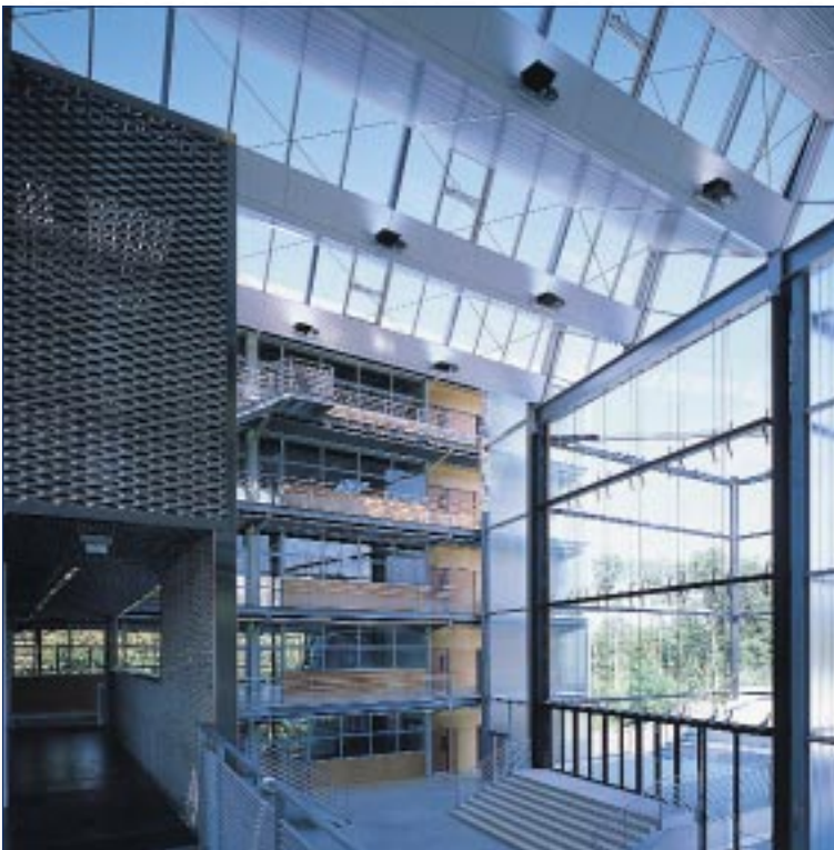
The Marne-la-Vallée School of Architecture (architect: Bernard Tschumi) puts three main materials on display: concrete, treated in various ways and left visible, metal, spread or diamond-tip cut, and glass for the façades and the roof.
