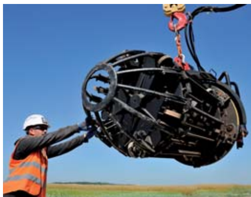
Clamping system on the Arc de Dierrey project, France.
