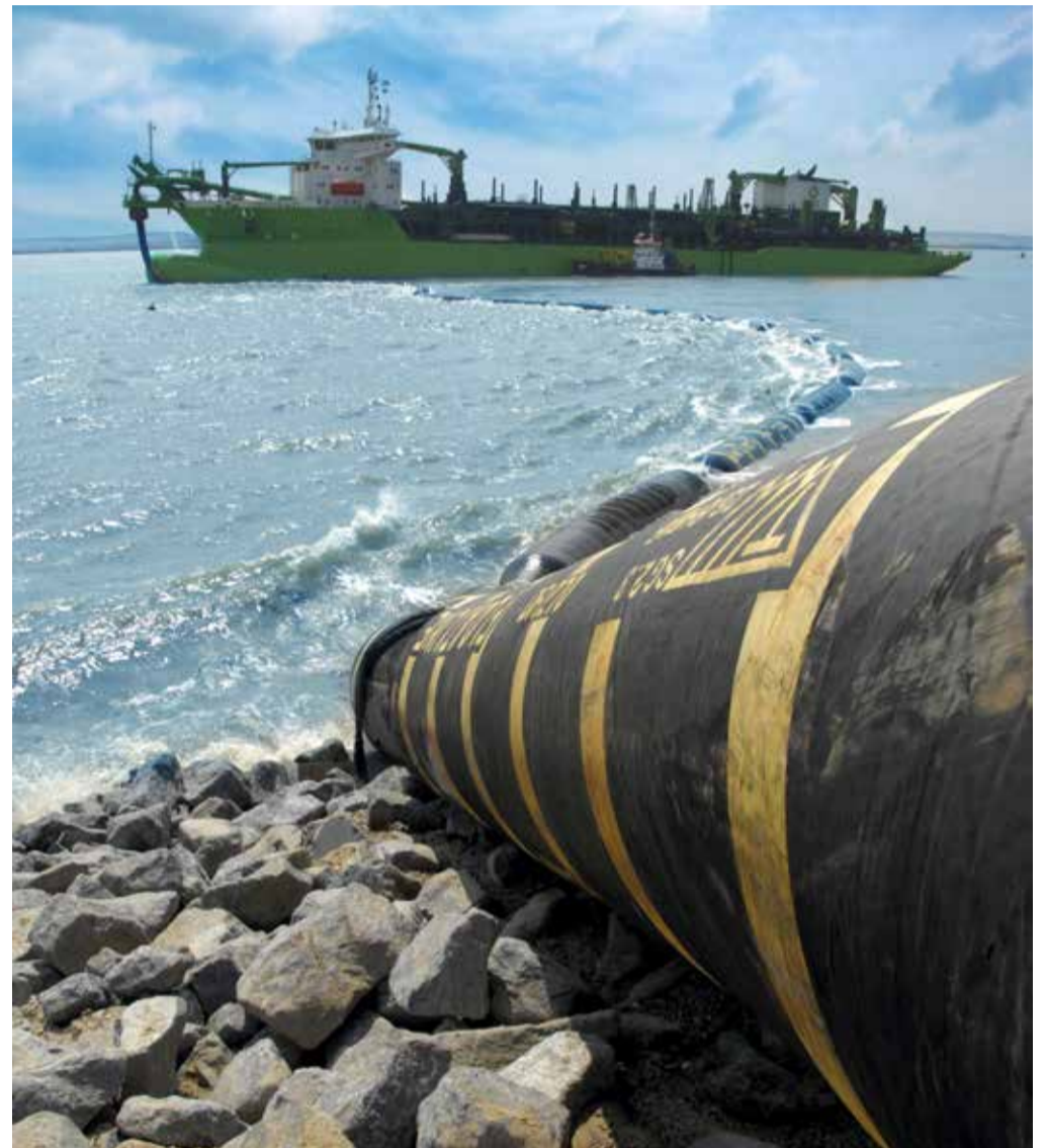
▲ Trailing suction hopper dredger Congo River - London Gateway project (UK)
