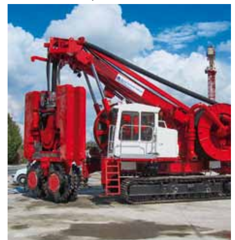
HC05, the new small Hydrofraise machine.
