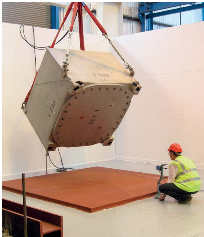
Impact resistance test at the VINCI Construction UK Technology Centre, where all sorts of tests are performed, from waterproofing of curtain walling to identification of building pathologies.
