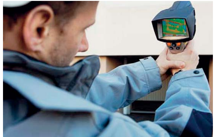
Thermal measurement during insulation works.
