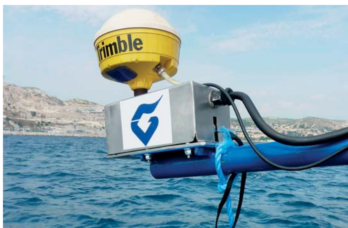
Developed by GEOCEAN (ENTREPOSE Contracting), this automatic buoy release system facilitates the precise location of mines during port de-mining operations.
