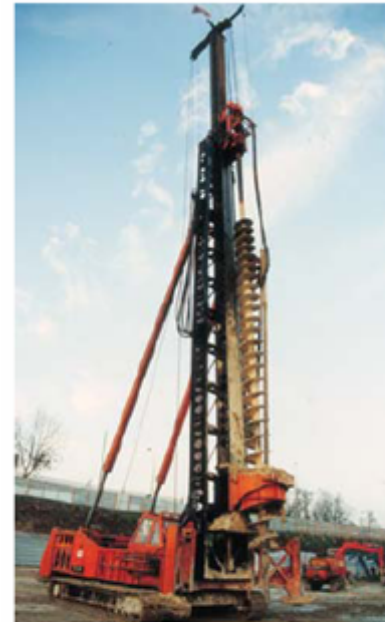
STARSOL - Continuous earth auger with integrated temie pipe and continuous recording of parameters
