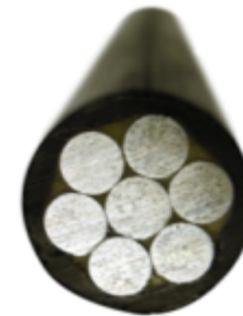
Freyssinet: “Cohestrand®: a solution for stresses in suspension bridge load-bearing cables”
